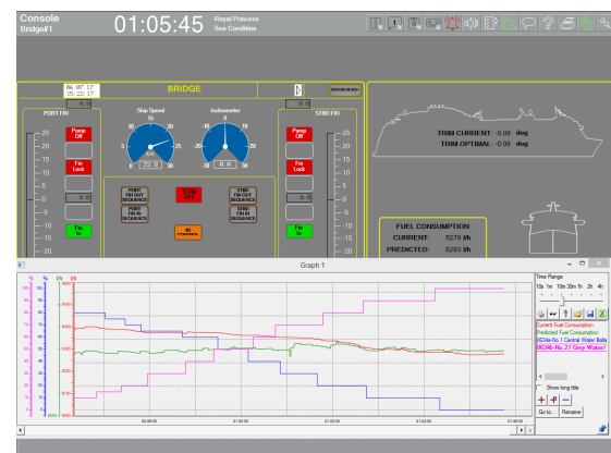
Figure 5. Speed and Fuel consumption after predicted trim applied
