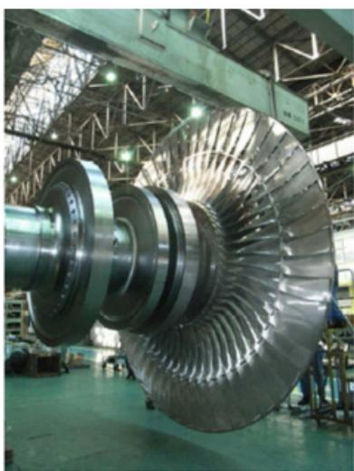
**Figure 3. The LP turbine last stages.**
