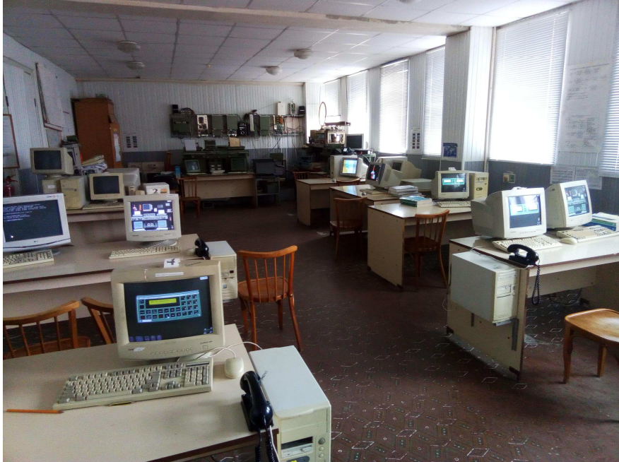
Picture 1. GMDSS simulator TGS-2000, 10 places+instructor
