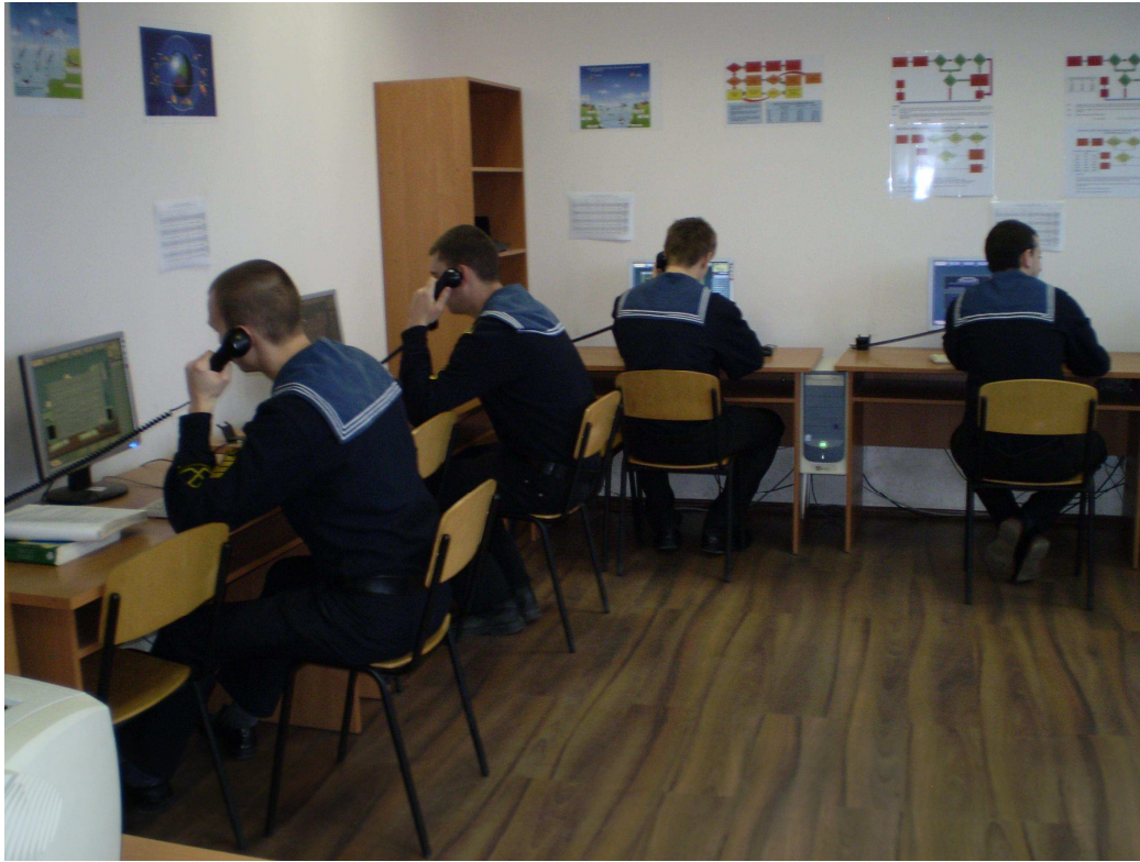
Picture 1. GMDSS simulator TGS-4100, 8 places+instructor
