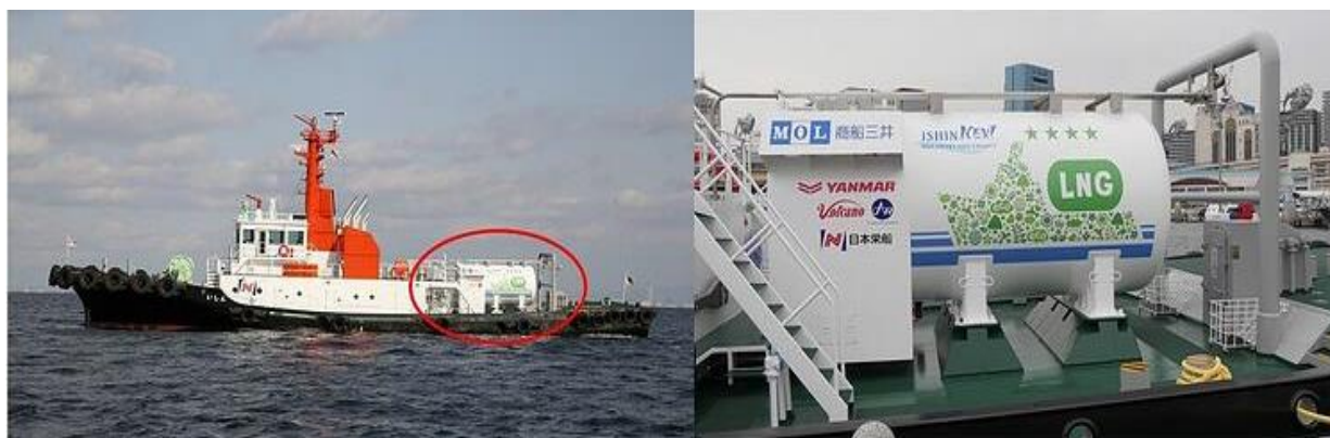
Fig. 1. Left: "Ishin" – tugboat operating on LNG; right: LNG tank on board the vessel.
