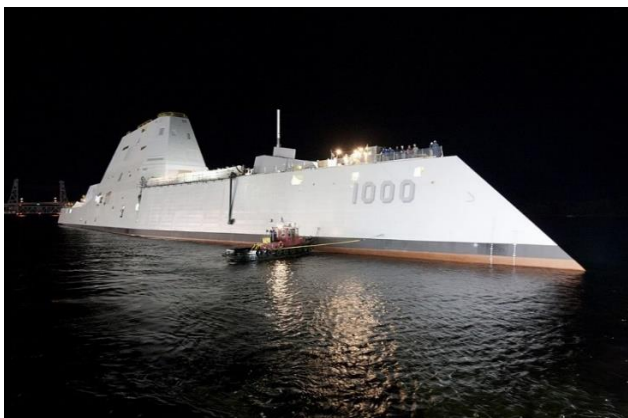
Fig. 3. American destroyer type "Zamvolt", made by stealth technology with a nose X-BOW, 2016
