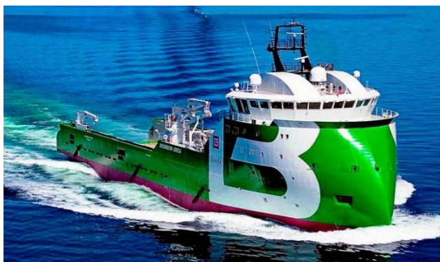
Fig. 1. Ship "Bourbon Orca" with technology X-BOW, 2006
